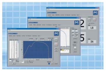
The program includes a set of tools to analyze test results, including statistical calculations, quick data export to Microsoft Excel, customizable reports, pass/fail indicators, and many others. Test setups and sequences are customizable and can be saved and recalled. The user can program test start and stop conditions, including load, time, distance, and sample break.
