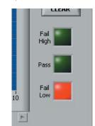
High and low limit indicators help differentiate between an acceptable sample and a reject
