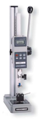
The TSB is shown in a wire terminal pull testing application, with a Series BG force gauge, wire terminal grip, and dual roller grip.
