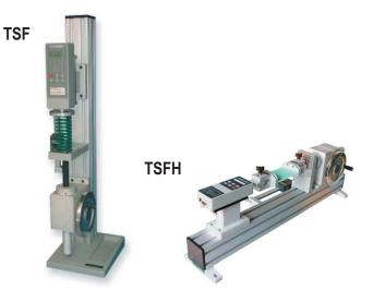
The TSF is shown testing the peel force of a sample, with a Series CG digital force gauge and digital travel display The TSFH is shown in a tensile test, with Series BG digital force gauge, film and paper grips, and digital travel display
